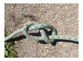
**<u>Timber hitch</u>** A timber hitch can be used to drag, lift or pull heavy equipment or logs. It can also be used as a base knot for lashing things together.
